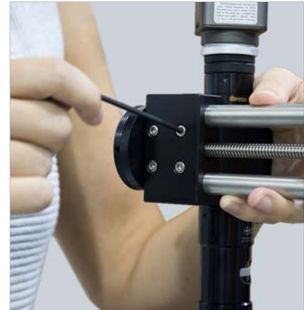
FIGURE 3-18 Left: Installing the microscope vertical post; Middle: Four M3 mounting screws on the vertical post; Right: Attaching the microscope to the horizontal boom
