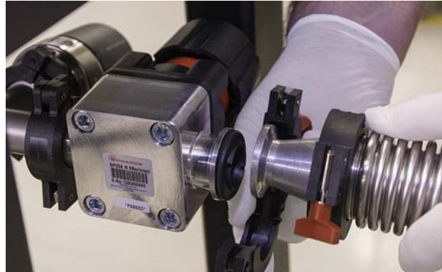
FIGURE 3-26 Use the clamp provided to attach the vacuum line to the Model CRX-6.5K probe station
