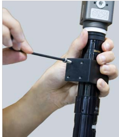
FIGURE 3-18 Left: Installing the microscope vertical post; Middle: Four M3 mounting screws on the vertical post; Right: Attaching the microscope to the horizontal boom
