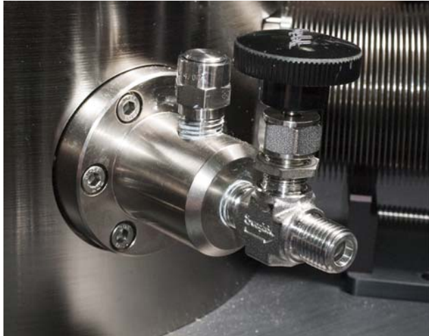
FIGURE 4-9 Left: Purge valve; Right: Vacuum isolation valve
