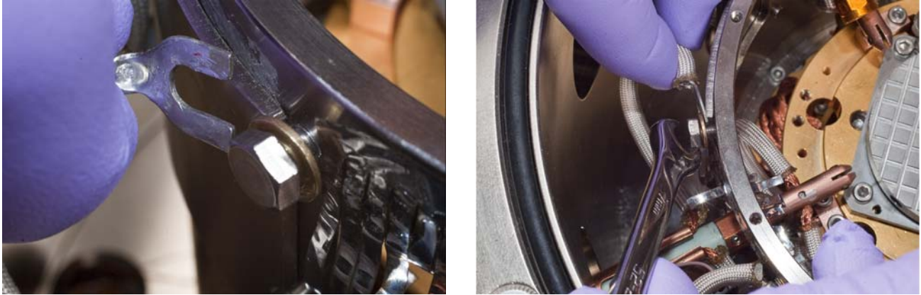
FIGURE 5-8 Left: Slide the spade lug under the hex screw head and washer; Right: Tighten the hex screw
