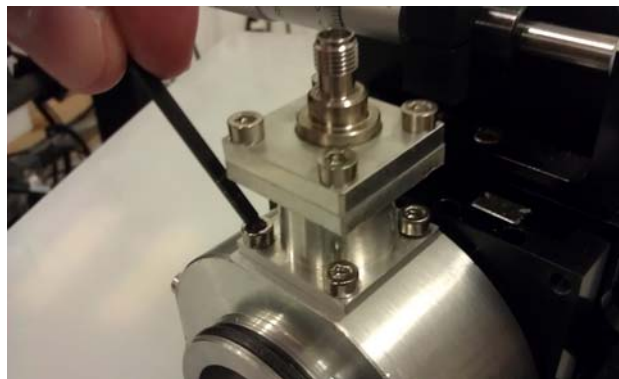
FIGURE 5-19 Remove the bottom set of four M3 screws
