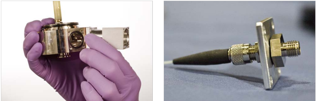
FIGURE 5-23 Left: Attaching the feedthrough extension to the probe arm base; Right: The nut between the cable and the flange—SMA style shown
