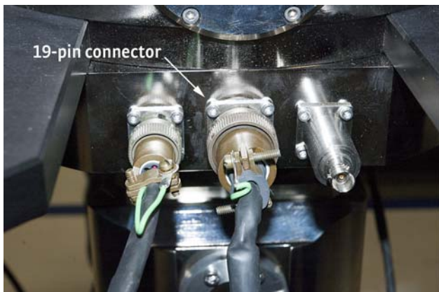
FIGURE 3-16 Left: Cable connection point at the back of the vacuum chamber for the sample and radiation shield thermometry; Right: Cable connection point at the side of the vacuum chamber shroud
