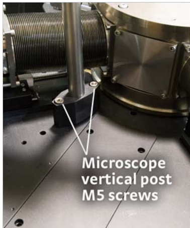
FIGURE 3-18 Left: Installing the microscope vertical post; Middle: Four M3 mounting screws on the vertical post; Right: Attaching the microscope to the horizontal boom
