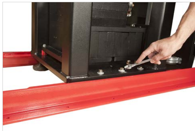
FIGURE 3-7 Removing the cross braces
