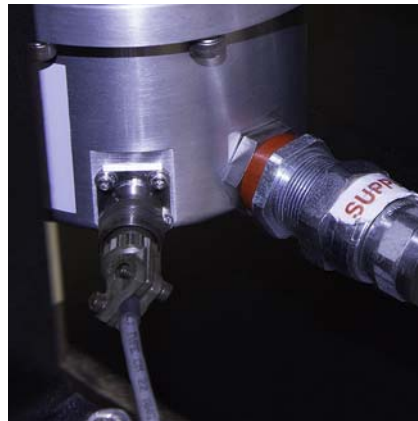
FIGURE 3-15 Left: Connect the cable to the cold head; Right: Connect the cable to the compressor
