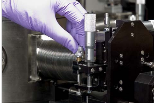
FIGURE 4-13 Turn the differential knob to adjust the angle
