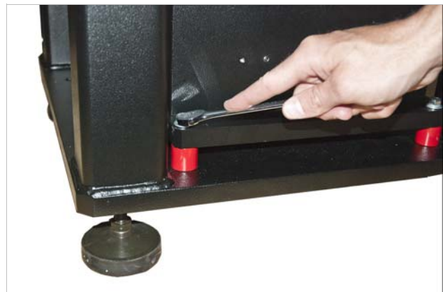
FIGURE 3-10 Left: Vibration isolation pads positioned under the CCR stand feet; Right: Remove the locking bolts and red spacing washers
