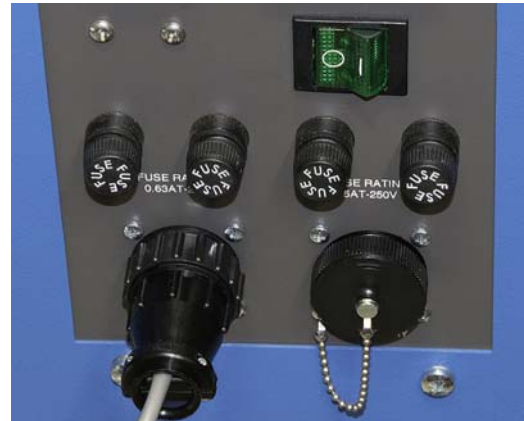
FIGURE 3-15 Left: Connect the cable to the cold head; Right: Connect the cable to the compressor
