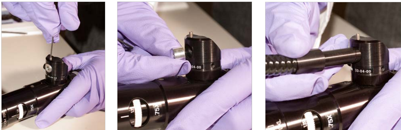
FIGURE 3-22 Left: Loosen the set screw on the fiber optic cable fitting; Middle: Remove protective fitting; Right: Insert the fiber optic cable
