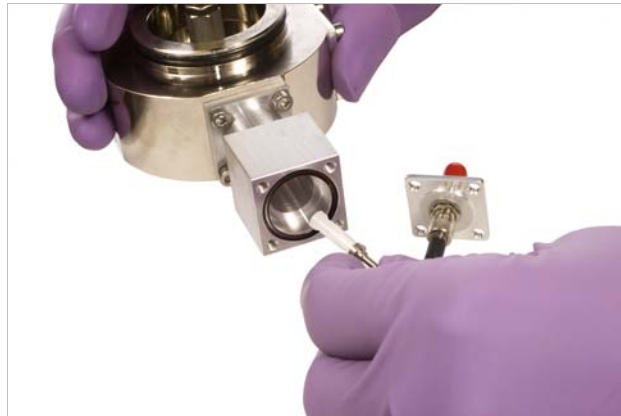
FIGURE 5-24 Insert the optical fiber tip into the feedthrough extension
