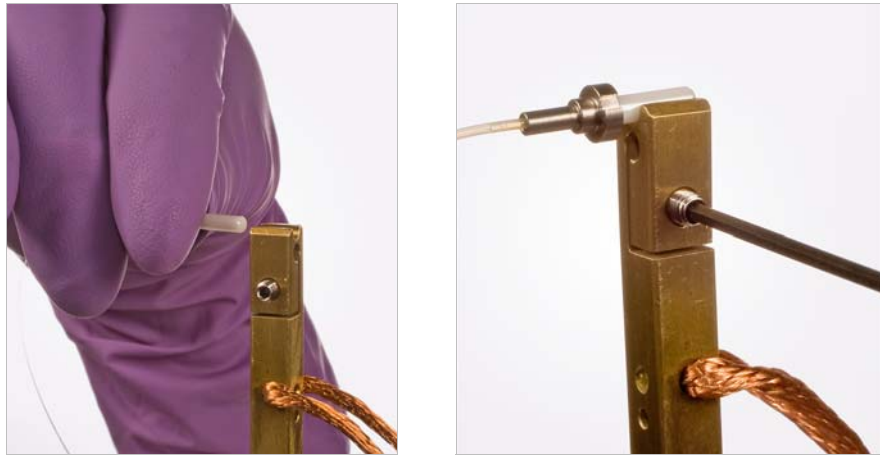
FIGURE 5-25 Left: Inserting the optical fiber tip into the opening in the probe mount; Right: Securing the optical fiber tip by tightening the M3 screw
