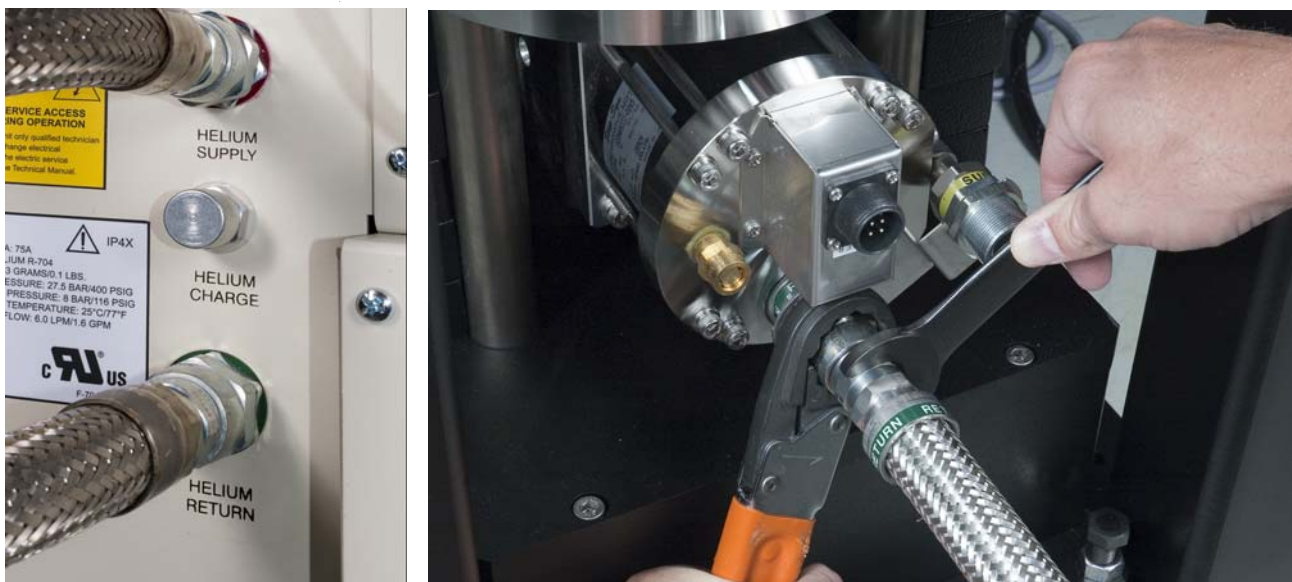
FIGURE 3-13 Left: On the compressor, connect the return line first, and then connect the supply line; Right: On the cold head, connect the return line first (shown) and then connect the supply line
