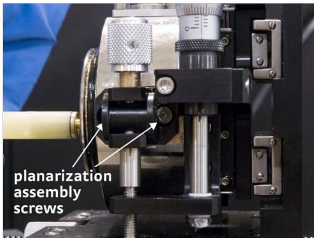
FIGURE 5-15 Left: Securing the planarization assembly to the probe arm base; Right: Taping the cable to the probe arm
