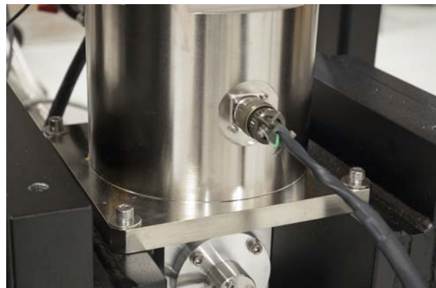
FIGURE 3-16 Left: Cable connection point at the back of the vacuum chamber for the sample and radiation shield thermometry; Right: Cable connection point at the side of the vacuum chamber shroud
