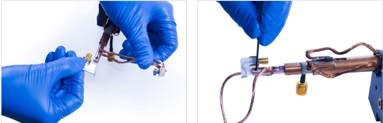
FIGURE 3-32 Left: Slide the blade into its slot; Right: Carefully tighten the probe mount set screws
