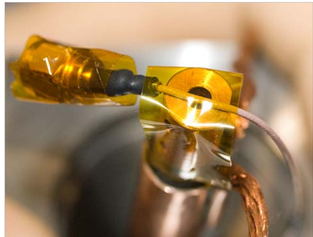
FIGURE 5-15 Left: Securing the planarization assembly to the probe arm base; Right: Taping the cable to the probe arm
