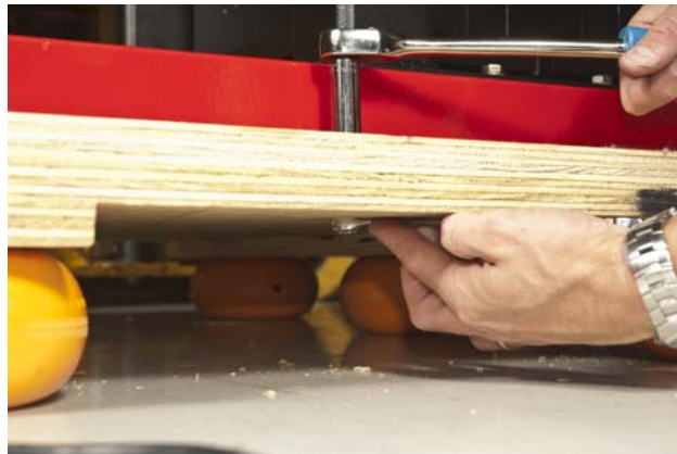
FIGURE 3-5 Remove the bolts attaching the red, horizontal cross braces to the crate base
