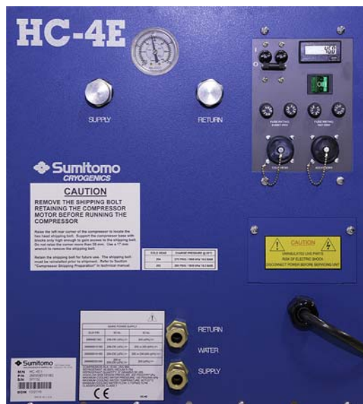
FIGURE 4-10 CCR compressor panel
