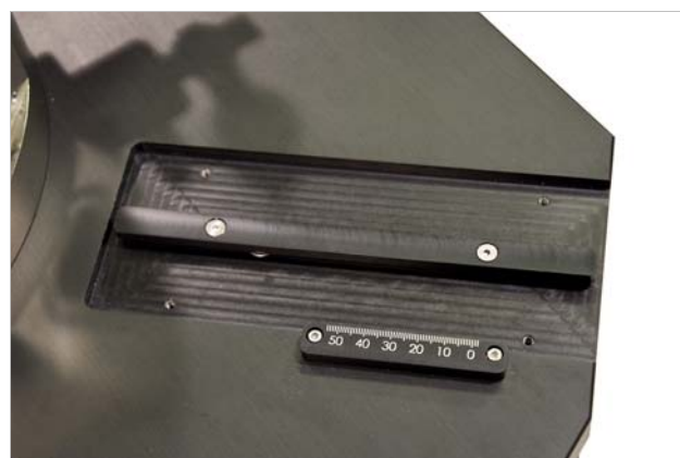
FIGURE 5-5 Left: Remove the screws from the slide insert; Right: Secure the slide insert to the arm stage location
