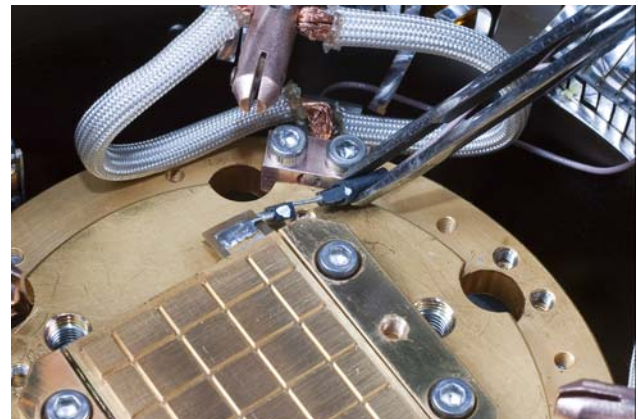
FIGURE 4-6 Left: Fastening the sample holder onto the sample stage; Right: Connecting the signal cable on a triaxial or coaxial sample holder
