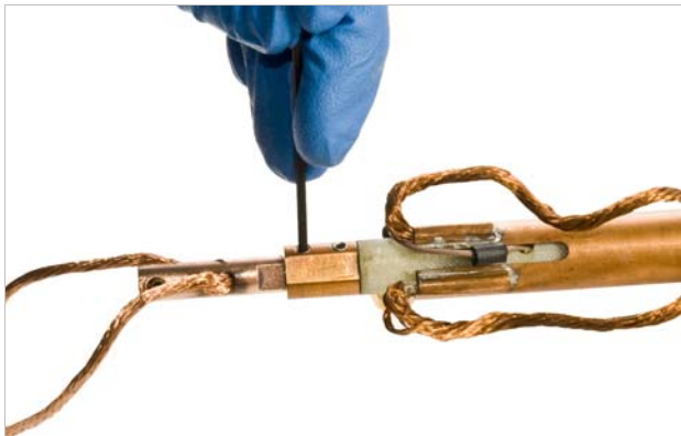
FIGURE 3-34 Loosen the probe arm set screws
