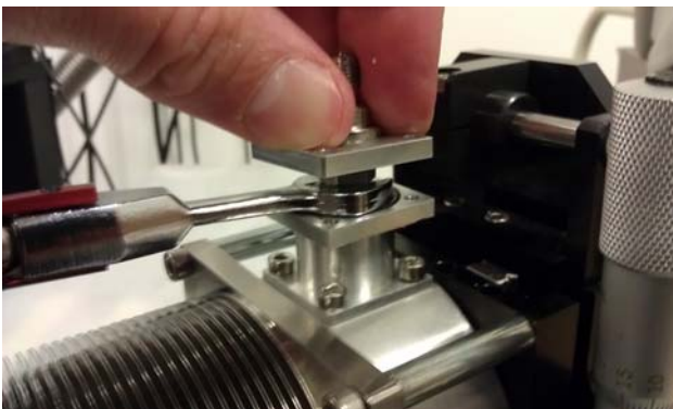
FIGURE 5-21 Left: Rotate the feedthrough assembly into position and re-tighten the connection; Right: The off-centered position on the cable feedthrough assembly
