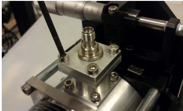
FIGURE 5-20 Remove the top set of four M3 screws
