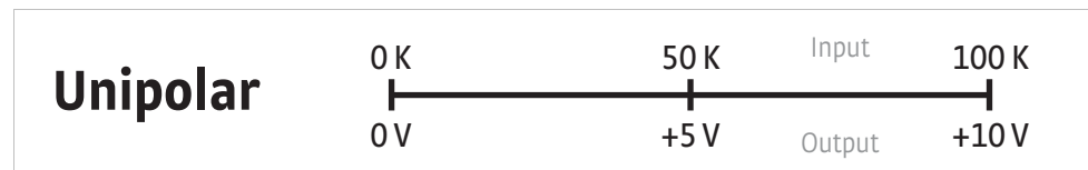
FIGURE 5-4 Output with polarity parameter set to unipolar
