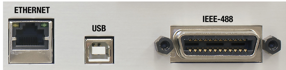
FIGURE 1-12 Ethernet, USB and IEEE-488 connections on the Model 372
