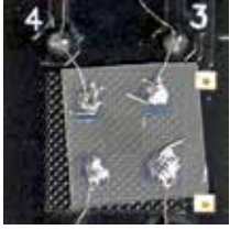
Typical Hall contacts eliminated by CRX-VF
