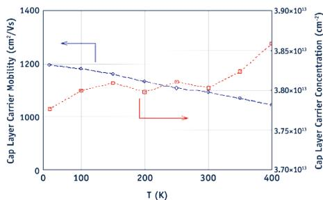
Analyzing the variable field and temperature data from a pHEMT sample, 2 electron carriers were identified at each temperature from 50 K to 400 K. The pHEMT sample was measured on the Model 9709A HMS.
