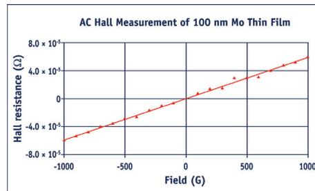
This measurement of Hall resistance vs. field for a 100 nm thick molybdenum thin film was taken while the sample was at a temperature of 50 K. The triangles are the measured data points and the line is the best-fit straight line. A change of resistance of  $10 \mu\Omega$  can easily be resolved. The measurement time is 20 s per point.
