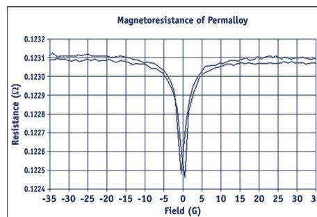
Lake Shore HMS can be used to characterize magnet-transport in magnetic materials. If the sample mount in an electromagnet system is rotated  $90^\circ$  so the field lies in the plane of the sample, classical MR measurements can be made. These MR measurements on a thin film Permalloy sample were taken on a Model 7704A system. Note that the small MR effect ( $\Delta R/R=0.5\%$ ) is easily seen. The small coercivity ( $\sim 1$  G) of the sample is also resolved.
