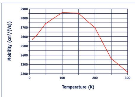
These figures demonstrate the mobility and density of Si as a function of temperature. The density is nearly independent of temperature and the mobility shows a typical electron-phonon scattering behavior.
