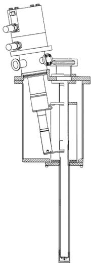
CCRs provide a variable temperature environment by cooling helium exchange gas. No liquid cryogenics are required, therefore, ongoing operating costs are minimal. The sample probe, rotation stage, and hose accessories are provided. The sample is surrounded by helium gas at a pressure slightly above atmospheric, so samples can be changed without breaking vacuum or warming up the CCR. Pump out of the vacuum jacket to 100 Pa (0.1 torr) is required before cooldown.
