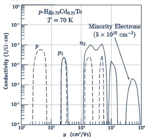
The structure of small bandgap materials like HgCdTe (used for near IR detectors) is very complicated, requiring high fields and variable temperatures to characterize. Using QMSA, this conductivity vs. mobility for a HgCdTe sample was taken with a Model 9709A HMS, which offers variable field capabilities to 9 T and a temperature range of 2 K to 400 K.
