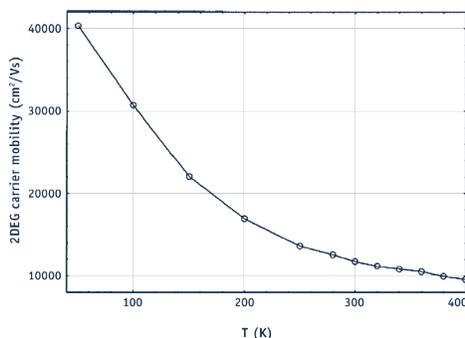
A typical pHEMT structure has a 2DEG high mobility carrier. A low mobility carrier associated with the cap layer is also often present. The mobility of high mobility carriers increases as temperature decreases. Using a variable field and temperature HMS along with QMSA®, the mobility of the 2DEG carriers can be distinguished from the cap layer carrier. This figure shows the temperature dependence of the 2DEG carrier mobility.
