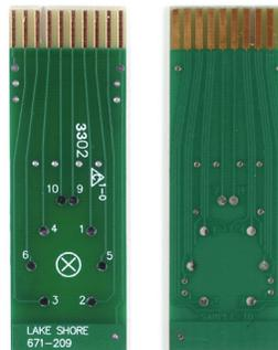
The 4-sample probe with two 2-sided plug-in sample cards facilitates consecutive multi-sample measurements without hardware exchange.
