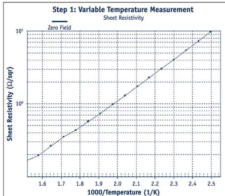
This figure shows the resistivity of germanium vs. temperature. The sample temperature varied from 400 K to 650 K. As expected, a log plot of resistivity vs. magnetic field to 1 T is a straight line.
