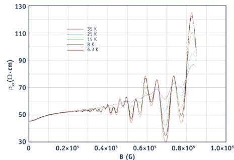
The SdH effect, mostly seen at low temperatures, is an oscillation of the magnetoresistance. Shown are SdH data for an InP pHEMT that was acquired with a Model 9709A HMS.
