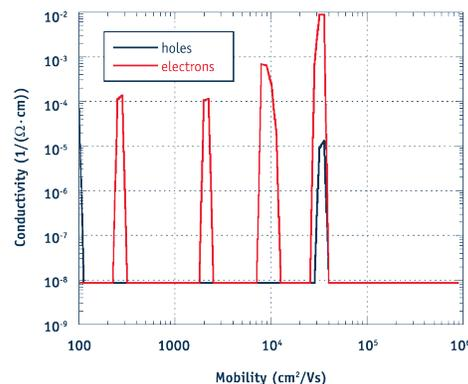
This is the resulting QMSA spectrum for a pseudomorphic high mobility transistor (pHEMT) structure. There are 4 distinct electron carriers and a single hole that populate this heterostructure device. The multi-carrier mixed conduction of this sample is clearly shown.
