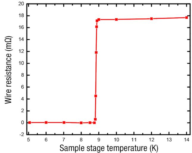
Figure 3—Superconducting transition in a probed niobium wire
