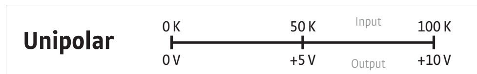
FIGURE 5-5 Output with polarity parameter set to unipolar
