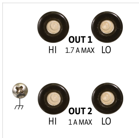
FIGURE 3-8 Rear panel showing heater output connectors
