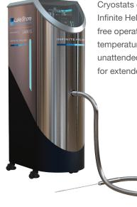
Cryostats can be combined with Infinite Helium for fully cryogenfree operation throughout the entire temperature range. This enables unattended cryostat operation, ideal for extended duration measurements.
