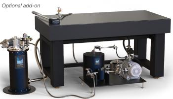
Cryostats can be combined with the RGC recirculating gas cooler for fully cryogen-free operation throughout the entire temperature range. This enables unattended cryostat operation, ideal for extended duration measurements.
