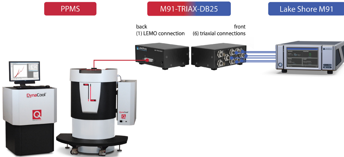
Diagram 1: PPMS connected to the M91 via breakout box
