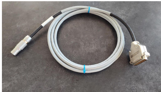
Lake Shore DB25 to LEMO cable (PN 112-819) with separated source to measure connections (left table pin map, below)
